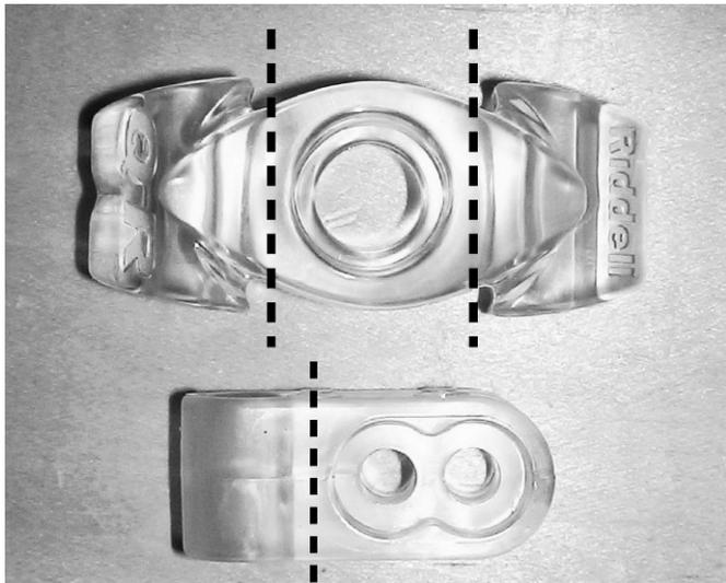
**Figure 9.** The Quick Release (Riddell Inc, Elyria, OH) loop strap requires 2 cuts, so approximately twice the amount of material needs to be cut compared with a traditional loop strap.
