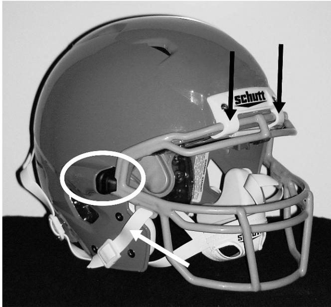
**Figure 6.** The ION 4D (Schutt Sports Inc, Litchfield, IL) helmet. The black arrows point to the locations on the face-mask retainer clip that need to be cut. The white arrow indicates the approximate location where the chin strap needs to be cut on both sides. The face mask inserts into the channels on each side of the helmet (white circle) and slides out when the chin straps and retainer clip are cut.
